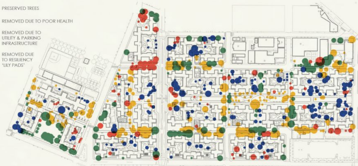
Figure 9. Tree removals at Red Hook enabled the construction of a continuous, passive flood protection system but required extensive tree removals.
